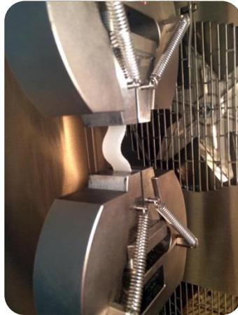
**Figure V.16.** Buckling of PLA-BS blend during DMA test at 30 Hz and 60 °C
