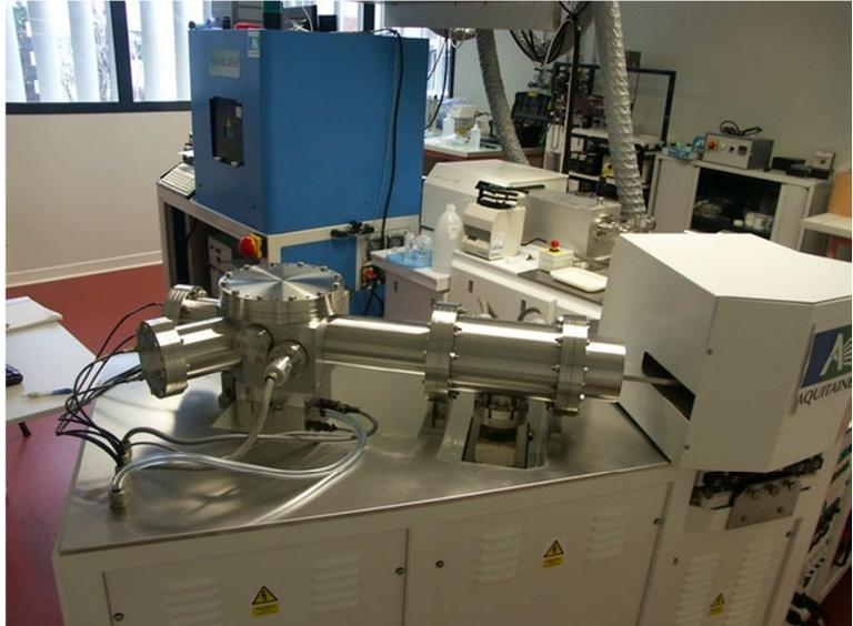
Figure 21 Couplage laser et MC-ICP-MS (© C. Pécheyran- LCABIE)
