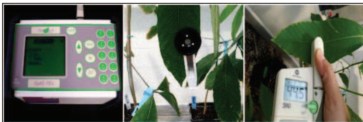
Figure 33. Instruments of chlorophyll fluorescence measurement.
