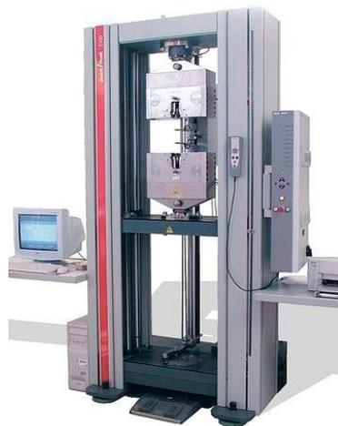
Figure 4.10 : Machine de traction ZWICK Roell 10kN.
