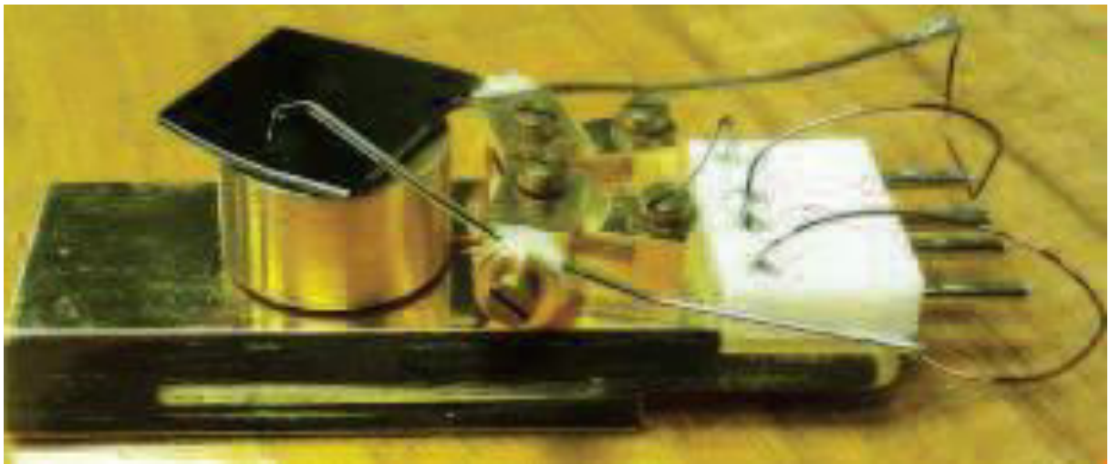
Figure E.4: Advanced EBIC sample holder with two probes.
