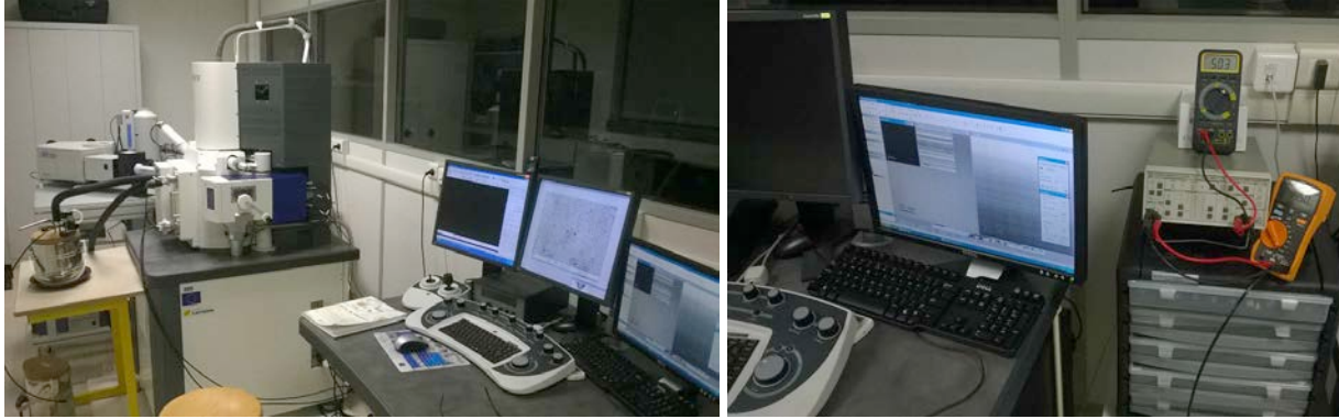
Figure E.3: EBIC setup used for the measurements in this thesis.
