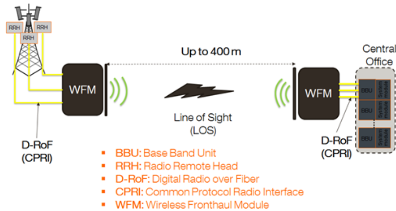
Figure 1.35: Architecture of wireless Fronthaul
