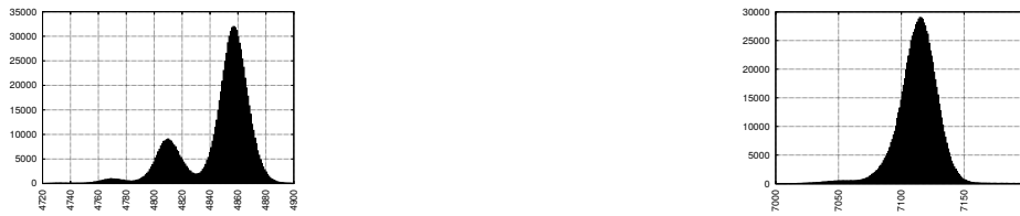
Figure 10.6: Illustration of two examples of distributions of the measured number of cycles (X-axis) of two different plaintexts during N runs of the AES encryption. The Y-axis refers to the number of times a given number of cycles has been represented among the N runs. The figure on the right has an execution time 1.75 times higher than the left one.
