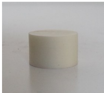
Figure 42: Characterization of the Zirconia material - 4GHz resonator
