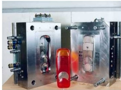
Figure 30: example of mold for injection [34]
