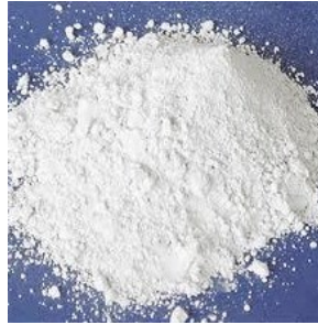
Figure 41: powder of Zirconia (Zirconium oxide)
