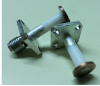
Figure 153: coaxial probe for the new Input/Output system
