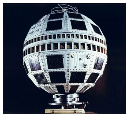
Figure 2: Telstar 1 : the first active satellite and commercial payload
