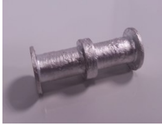
Figure 186: 2-pole dielectric part covered by silver lacquer
