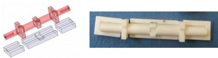
Figure 134: designed and manufactured dielectric part of the filter with support
