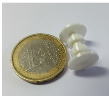
Figure 182: Manufactured dielectric part - 3-pole filter
