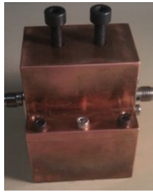
Figure 122: metallic housing for the 2-pole filter
