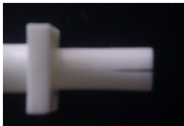
Figure 141: crack on the dielectric element of the 4-pole filter
