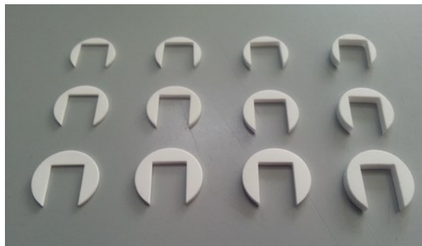
Figure 164: a set of dielectric rings for the 2-pole filter with tuning
