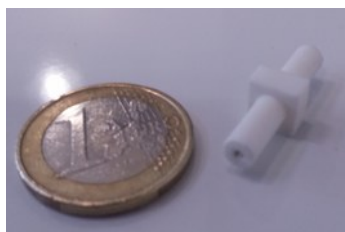
Figure 119: dielectric part of the 2-pole filter
