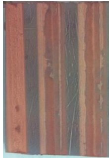
Fig. 68 Trial of deposition additional tracks to form a coating
