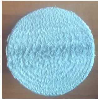
Fig. 49 View of cohesive type of fracture after adhesion test.
