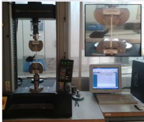
Figure II. 13 : Essai de traction (INSTRON 5567)
