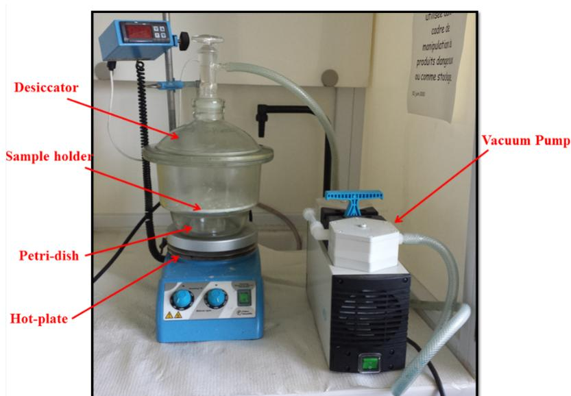
Figure 3.4 – **Schematic set-up of silanization procedure.** Vapor phase deposition of PFOTS by increasing the percent partial pressure of the organosilane within a close chamber (desiccator).
