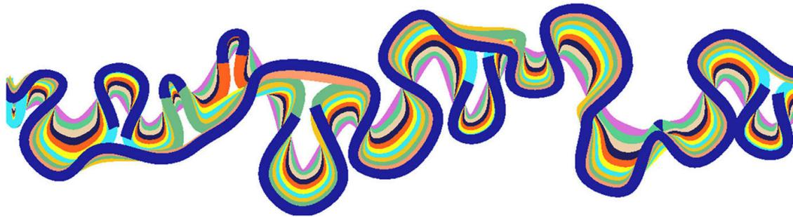
**Fig. 22** Result of the oxbow lake formation during the channel lateral migration
