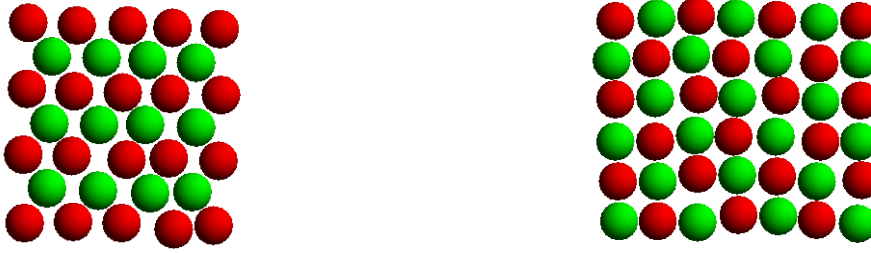
Figure 4.8: The arrangement of first layer of colloids at the surface of the wall. The CsCl structure (left) has its (101) plane attached at the surface of the wall while the NaCl structure (right) has its (100) plane attached at the surface of the wall. The two kinds of arrangements lead to P_{2D} values of different signs.
