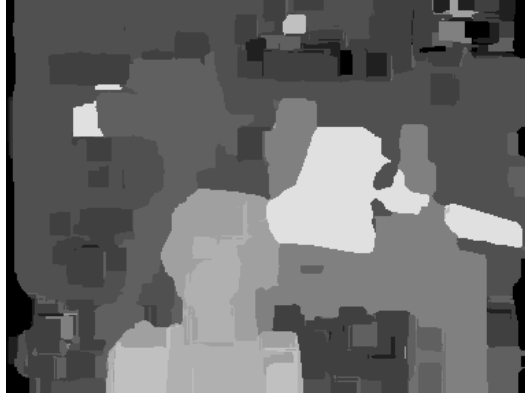
Figure 3.5: Disparity map computed by shiftable window approach.
