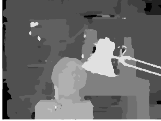
Figure 3.21: Disparity map computed by minimum spanning tree based ASW approach.
