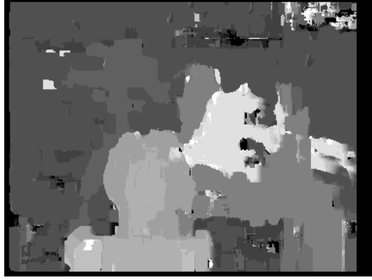
Figure 3.2: Disparity map computed by normalized cross-correlation.
