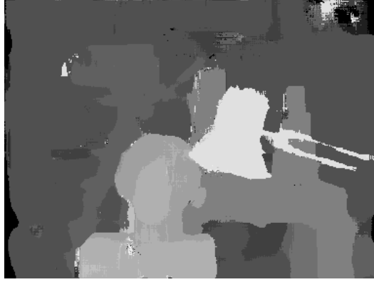
Figure 3.27: Disparity map computed by geodesic diffusion based ASW approach.
