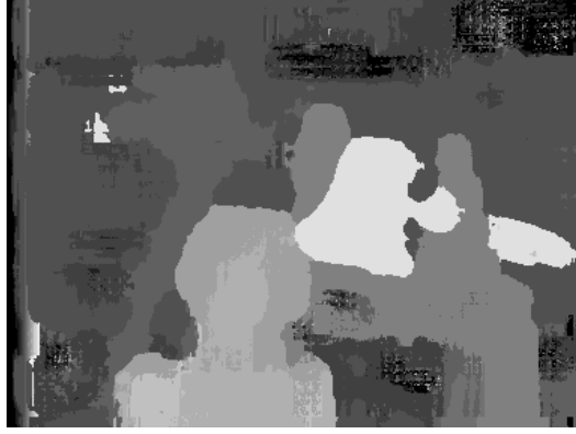
Figure 3.9: Disparity map computed by multiple window approach.
