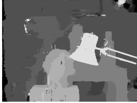
Figure 3.28: Disparity map computed by guided filter based ASW approach.
