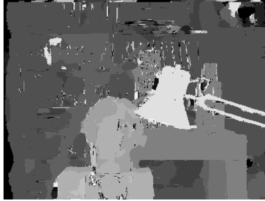
Figure 3.23: Disparity map computed by geodesic weight based ASW approach.
