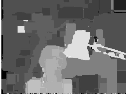
Figure 3.13: Disparity map computed by variable window approach.
