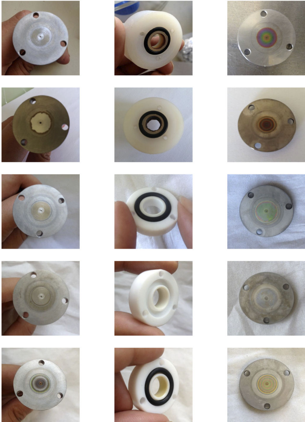
Figure 2.9: Picture of deposits for different insulator materials and under different gas flows. From left to right: Cathode; insulator; anode after a run of six hours. 1 st raw: Air flow and Nylon; 2 nd raw: Air flow and Nylon with silica gel ceramic coating; 3 rd raw: Air flow and Teflon; 4 th raw: Argon flow and Teflon; 5 th raw: Nitrogen flow and Teflon.
