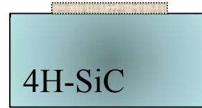
Figure 3.4 Definition of the implantation zone by photoresist
