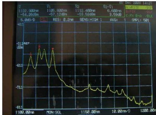
Figure 1: Fluorescence of Nd :YAG in the  $1100\text{--}1200\text{ nm}$  window
