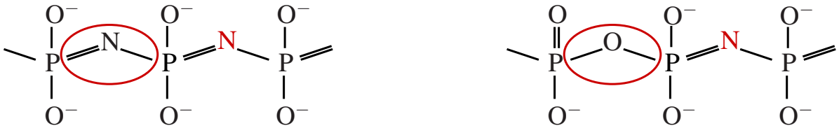
FIGURE 3.5 – Schematic representation of the effects, on the second coordination sphere around a nitrogen atom (in red), of a chemical modification : (left) \text{Li}_2\text{PO}_2\text{N} and (right) \text{Li}_{1.5}\text{PO}_{2.5}\text{N}_{0.5}
