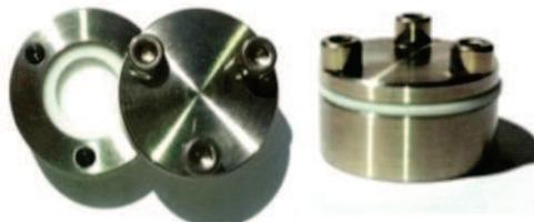
Figure 5.3 SCHEMA DU MOULE CASTING POUR POLYMERISER LA BORAZINE EN POLYBORAZYLENE.
