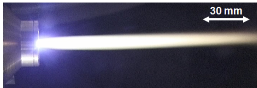
Figure 3.11: Laminar feature of pulsed arc jet. Operating parameters: d_{\text{nozzle}} = 4 \text{ mm} , I = 15 \text{ A} , N_2: 0.042 \text{ g.s}^{-1} , \bar{U} = 73.7 \text{ V} , exposure time of camera = 10^{-2} \text{ s} , the superposition of 13 cycles presented in Figure 3.10 [74].
