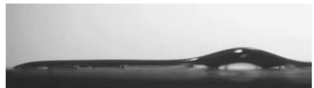
Fig. 14 Bulge formation in a microchannel
