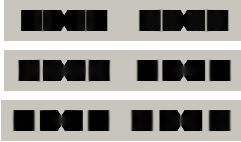
Figure 5.7: The plate breaking dynamics is shown for V = \pm 100 \text{ m/s} for time instants 1.4 \times 10^{-3} \text{ s} , 2.7 \times 10^{-3} \text{ s} , 4.0 \times 10^{-3} \text{ s} , 5.4 \times 10^{-3} \text{ s} , 6.7 \times 10^{-3} \text{ s} and 8.3 \times 10^{-3} \text{ s}
