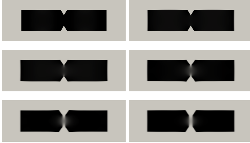
Figure 5.6: The fracture dynamics is shown for V = \pm 40 \text{ m/s} for time instants 1.8 \times 10^{-3} \text{ s} , 3.6 \times 10^{-3} \text{ s} , 5.4 \times 10^{-3} \text{ s} , 7.1 \times 10^{-3} \text{ s} , 8.9 \times 10^{-3} \text{ s} and 11 \times 10^{-3} \text{ s} .
