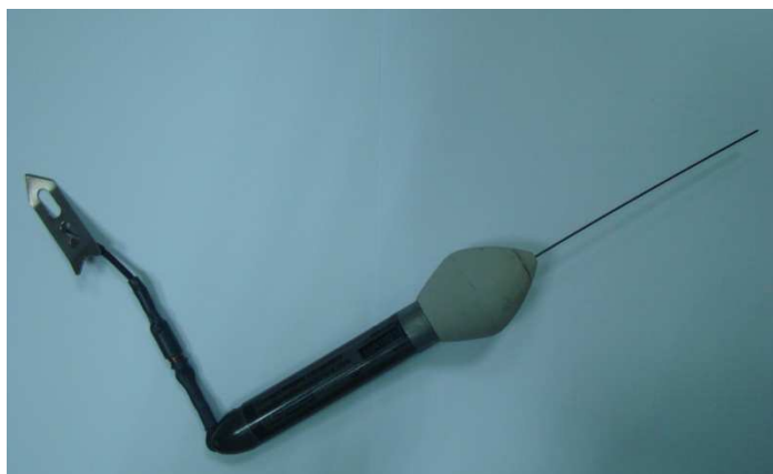
Figure 37 : Tag satellitaire Mk10-PAT tag (Wildlife computers)
