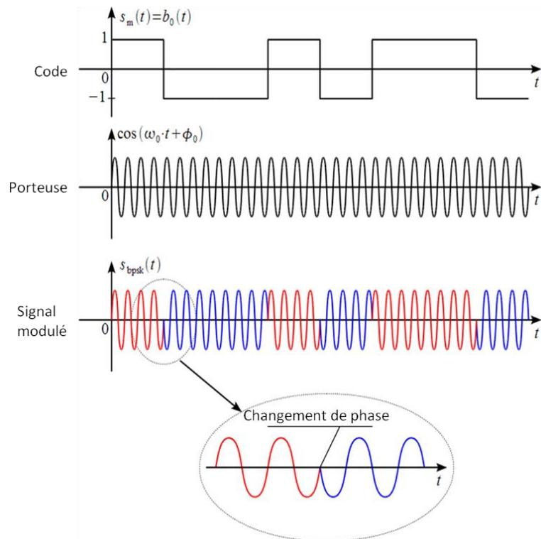
Figure I-4 : Modulation BPSK
