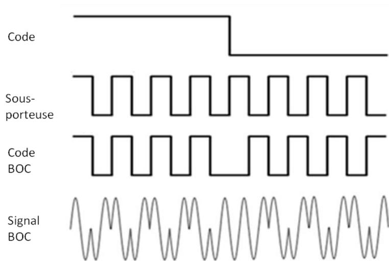
Figure I-5 : Modulation BOC
