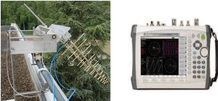
Figure 2. Mounting of the antennas on the roof and the VNA used for this experiment, respectively left and right.
