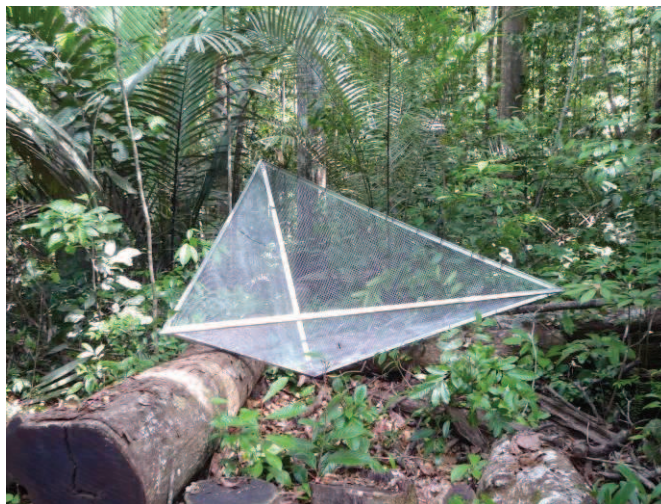
Fig. 3. Picture of the trihedral reflector.
