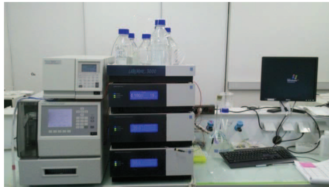
Figure I-8 : Chromatographe liquide haute performance (HPLC)
