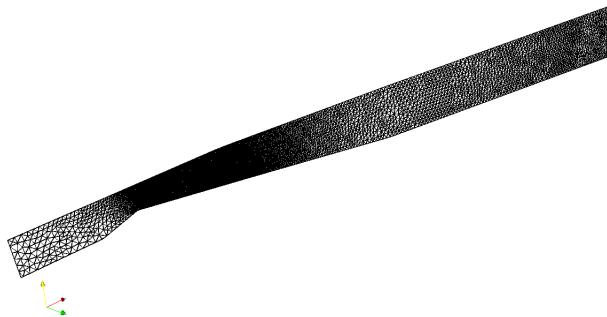
FIGURE 1.13 – Venturi  $8^\circ$  2D unstructured mesh.
