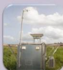
Figure 4. PAO Remtech Sodar in the landfill of La Gabarre
