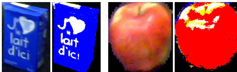
Figure 41: Two objects extracted from robot's surroundings. Right: the original image, left: features interpreted. For the “apple”, the robot's given description was “the object is red”. For the box, the description was “the object is blue and white”.
