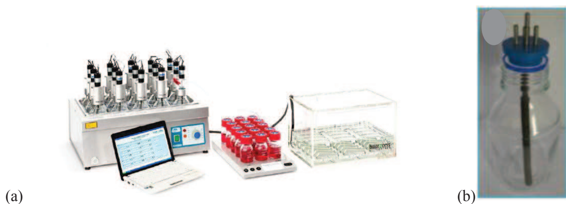
Figure 6 : (a) AMTPS from BIOPROCESS CONTROL and (b) glass bottle with stirring device
