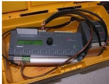
Figure III-2. Centrale d'acquisition IDL100
