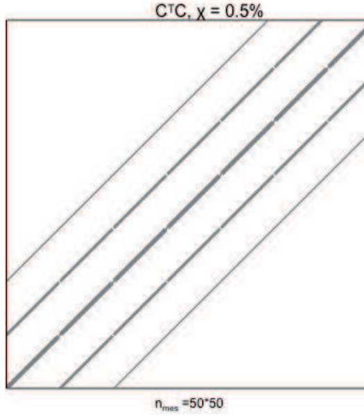
Figure 5.19: A sparse approximation of C_{kol}^{-1} represented for a grid of 50 \times 50 in the pupil of the telescope, the matrix is 0.5 % filled.
