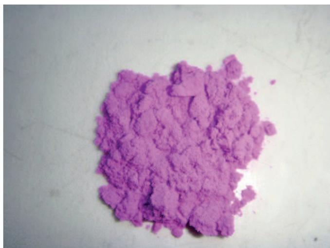
Figure 121 : Poudre de  $\text{LiMn}_{0,5}\text{Co}_{0,5}\text{PO}_4$
