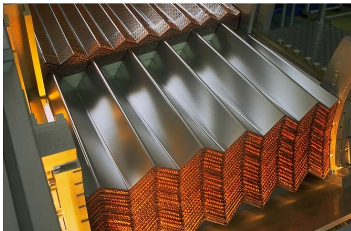
Figure 3.2: Photograph of barrel accordion-shaped electrodes and absorbers [83].
