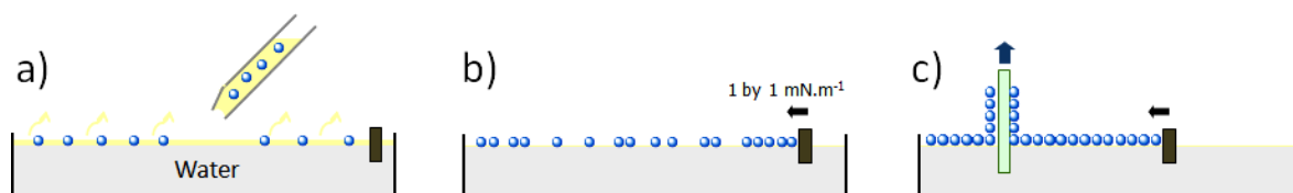
Figure 2.10: Different steps involved in the Langmuir-Blodgett process together with colloidal particles. a) Spreading of the particles on the water surface. b) Compression of the Langmuir film. c) Transfer of the colloidal film to a hydrophilic substrate at constant surface pressure
