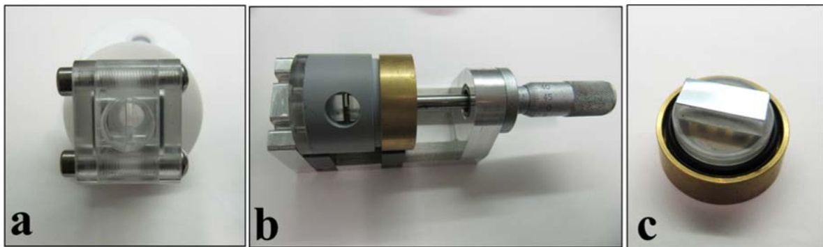
Figure II.22. (a) ZetaCAD cell with constant gap, (b) CRPP made cell with adjustable gap and (c) polystyrene coated silicon wafer sample (25mm×10mm) mounted on a cell component.
