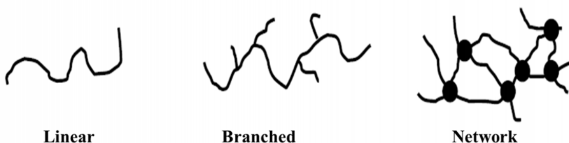
Figure I.5: Schematic architectures of different polymers.
