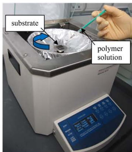
Figure II.3: G3 series Spin Coater (Specialty Coating Systems, SCS) and representation of the spin-coating technique for the deposition of a polymer film.
