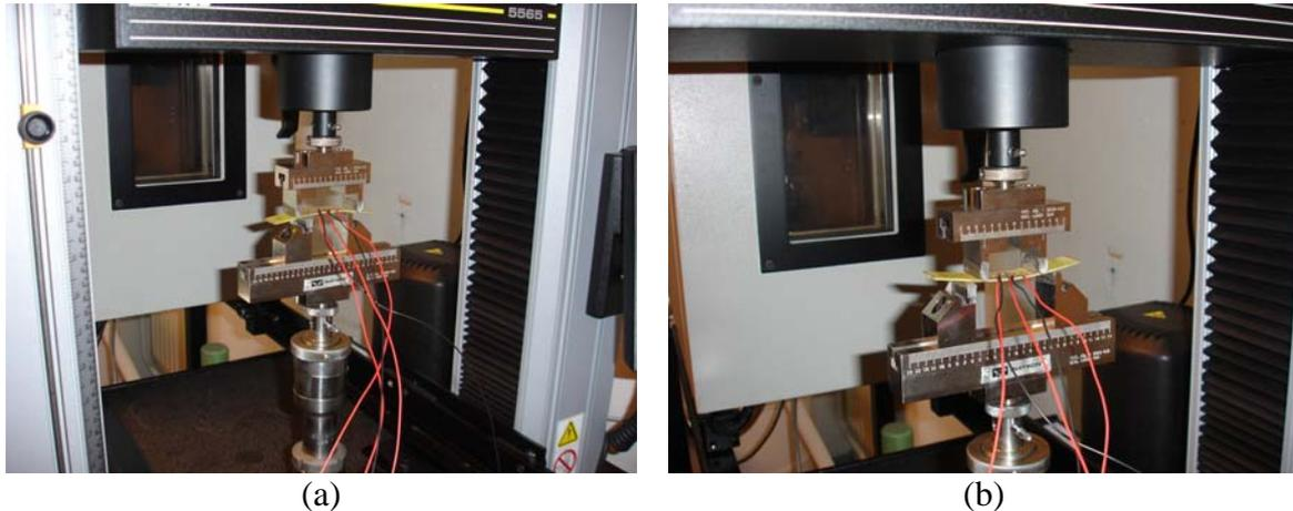
Figure 5.34 Substrat FR-4 sous flexion (a) Traction - Compression, (b) Compression - Traction
