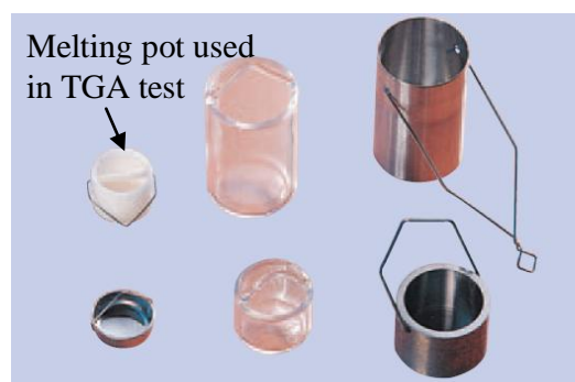
Figure 49. Some specific melting pots adapted to TGA (Thermogravimetric analysis) application
