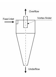
Figure II-1 A schematic diagram of a conventional cylindrical hydrocyclone
