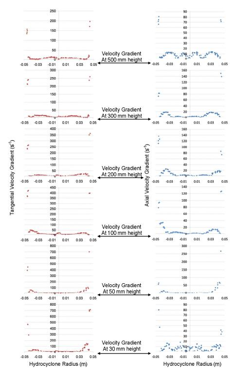
Figure V-8 Tangential and axial velocity gradients from Reynolds Stress Model numerical simulation at different level height (1000L/hr inlet flow rate, 1.572m/s inlet velocity)
