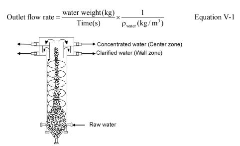
Figure V-3 Water zone for sampling for result analyzing
