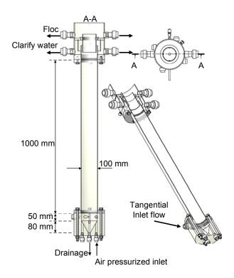
Figure III-4 Hybrid reactor dimension: Front, Top and Lateral views
