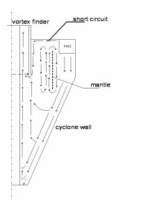
Figure II-3 A simplified diagram of the axial and radial flows in a hydrocyclone
