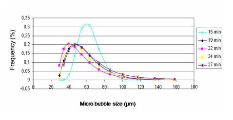
Figure IV-20 Reproducibility measurement experiment with 5.4bars saturated pressure
