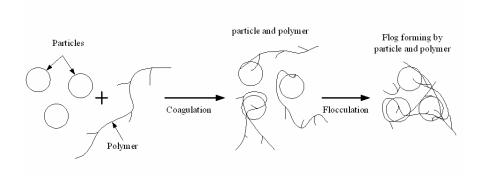
Figure V-33 polymer bridging mechanism
