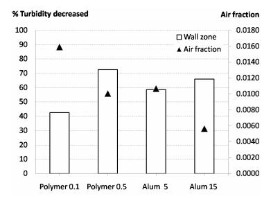
Figure V-13 %turbidity decreased and air fraction of 0.25g/L bentonite suspension with varied coagulant concentration without a static mixer
