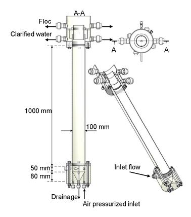
Figure V-2 Hydrocyclone reactor dimensions
