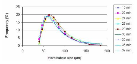
Figure IV-19 Reproducibility measurement experiment with 3.4bar saturated pressure
