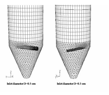
Figure IV-4Grid system of Hydrocyclone I with 0.5 and 0.3cm inlet diameter
