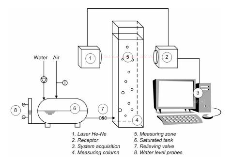
Figure IV-15 Schematic of the installation
