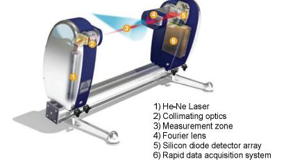
Figure III-1 Spreytec Malvern Instrument
