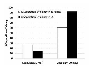
Figure V-30 % of separation efficiency comparing between 30 and 70mg/L coagulant concentration
