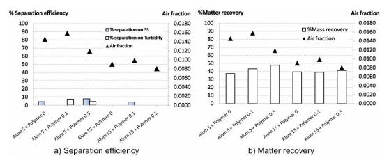
Figure V-17 separation efficiency and matter recovery fraction of 0.50g/L bentonite suspension with varied coagulant, flocculant concentrations with a static mixer (Pre coagulation)
