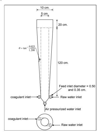
Figure II-16 Conical hybrid reactor size and details
