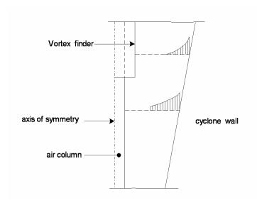
Figure II-6 Radial velocity distribution in a hydrocyclone
