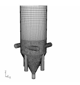
Figure IV-5 Grid system of Hydrocyclone II
