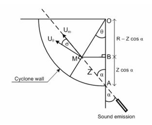
Figure IV-3 The Doppler method and the relation of the angle between the hydrocyclone diameter and the sound direction
