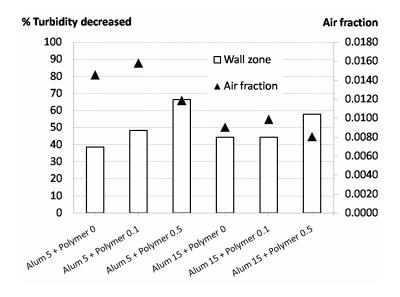
Figure V-14 %turbidity decreased and air fraction of 0.50g/L bentonite suspension with varied coagulant, flocculant concentrations with a static mixer (Pre coagulation)
