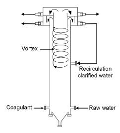
Figure V-38 The perspective sketch of hybrid reactor
