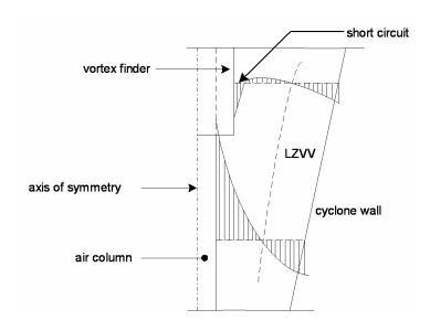
Figure II-5 Axial velocity distribution in a hydrocyclone. LZVV in the locus of zero vertical velocity
