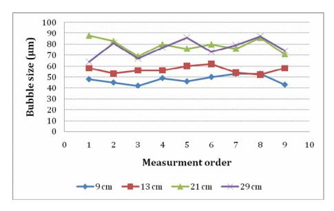
Figure IV-22 Micro bubble size from each height measurement (P=3 bar)
