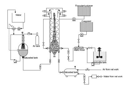
Figure V-11 Pilot schematic diagrams with static mixer
