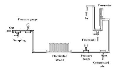
Figure II-10 The FF-flocculation-flotation system.
