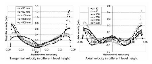
Figure V-9 tangential and axial velocities inside hydrocyclone at different height levels
