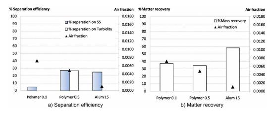
Figure V-15 Separation efficiency and %matter recovery fraction of 0.10g/L bentonite suspension with varied coagulant concentrations without static mixer
