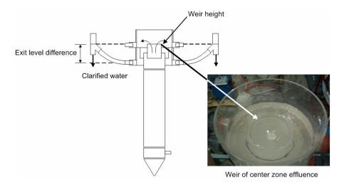
Figure V-27 Weir and the exit level difference
