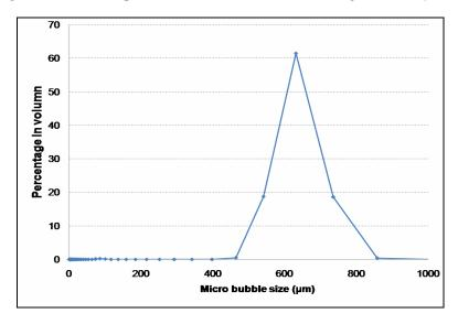
Figure IV-17 Volumetric percentage of bubble size
