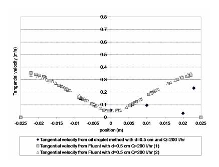
Figure IV-7 Tangential velocity with D= 0.5cm and velocity inlet 2.83 m/s
