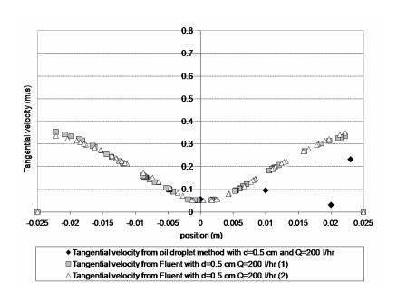
Figure IV-10 Tangential velocity with inlet flow rate 200L/h, velocity inlet 2.83m/s
