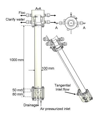
Figure V-20 Hydrocyclone reactor, front, upper and lateral view
