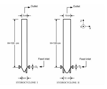
Figure IV-1 Schematic diagram of Hydrocyclone I ( $D_1$ =0.3 and 0.5cm) and Hydrocyclone II ( $D_2$ =1.5cm)
