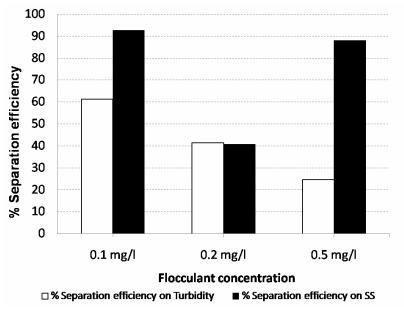
Figure V-34 Separation efficiency with a varied flocculant concentration
