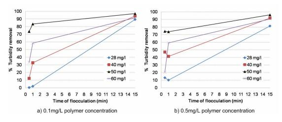
Figure V-22 The flocculation time and coagulant concentration affect on the % of turbidity removal
