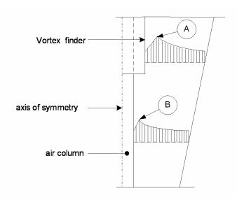
Figure II-4 Tangential velocity distribution in a hydrocyclone (V<sub>v</sub>)
