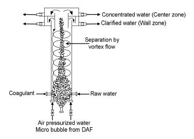
Figure IV-14 The hybrid reactor concept
