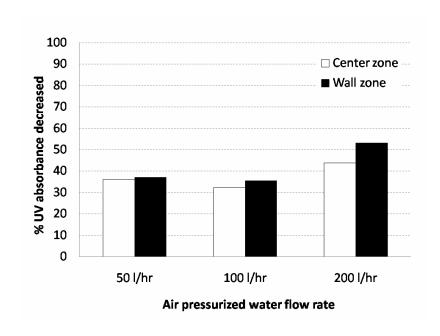
Figure V-35 The percentage of UV absorbance decreased with varied air pressurized water flow rates
