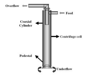
Figure II-11 The aerated floc flotation separator
