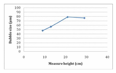
Figure IV-23 Average micro bubbles size from each height measurement
