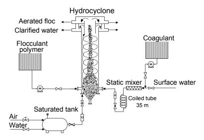
Figure V-19 Pilot plant schematic
