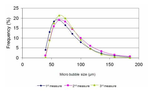
Figure IV-21 Reproducibility measurement experiment with 5.4bar saturated pressure
