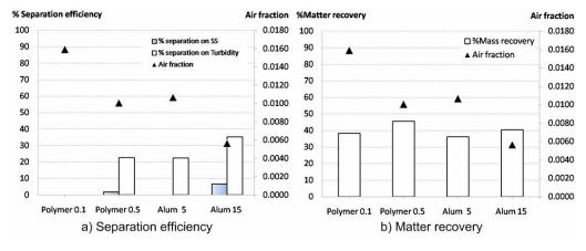
Figure V-16 separation efficiency and matter recovery fraction of 0.25g/L bentonite suspension with varied coagulant concentration without a static mixer
