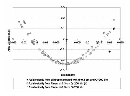
Figure IV-8 Axial velocity with D= 0.3cm and velocity inlet 7.86 m/s
