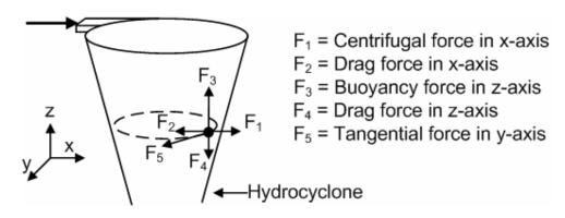
Figure II-7 Various forces applied on particle from different axes
