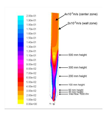
Figure V-7 the magnitude velocities in hydrocyclone from numerical simulation (1000L/hr inlet flow rate, 1.58m/s inlet velocity)
