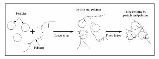
Figure II-9 Polymer bridging mechanism
