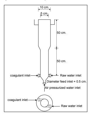
Figure II-15 Cylindrical hybrid reactor size and details
