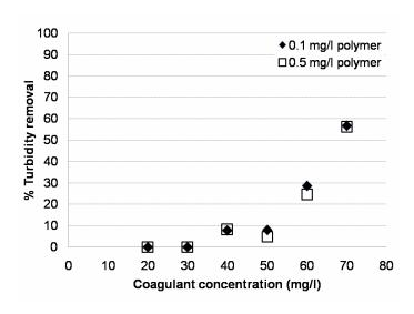
Figure V-25 Coagulant concentrations effect to turbidity removal percentage
