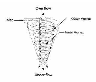
Figure II-2 A perspective view of a hydrocyclone showing the vortex flow inside schematically
