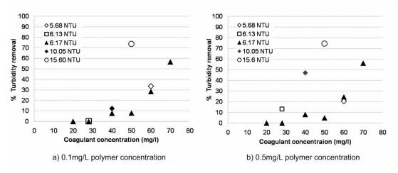
Figure V-24 The effect of raw water turbidity and turbidity removal percentages
