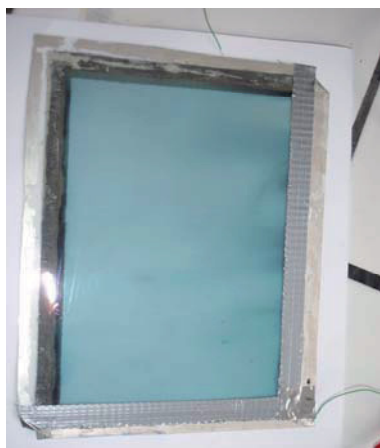
a) Bleached and colored states after 2 600 cycles between +1.0V and -1.3V
