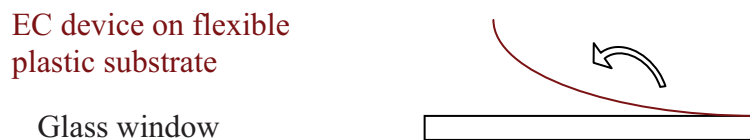
Figure I.5 : Illustration of the lamination of an EC device prepared on flexible plastic on a flat substrate. This substrate could be curved, flexible, etc.
