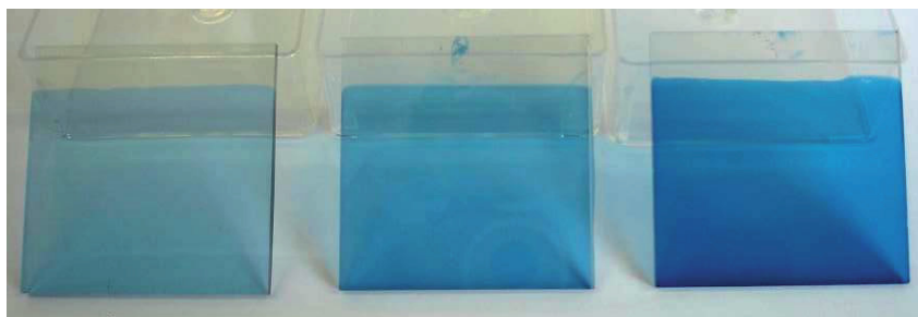
Figure III.20 : Prussian Blue films electrodeposited on FTO/glass ( R_{\Omega\Box} = 13 ) with capacities of 3, 6 and 12 \text{mC}/\text{cm}^2
