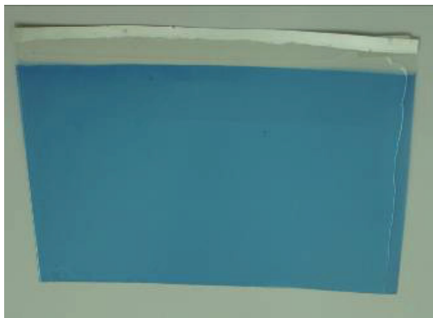
Figure IV.6 : Electrolytic membrane deposited on the Prussian Blue layer
