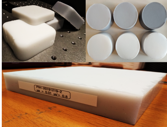
FIGURE 5.2: Silicone-based tissue mimicking phantoms manufactured and used for the validation of the multi-modal referencing platform.
