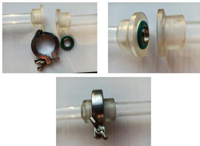
Fig. 2.6 Sealing joints.
