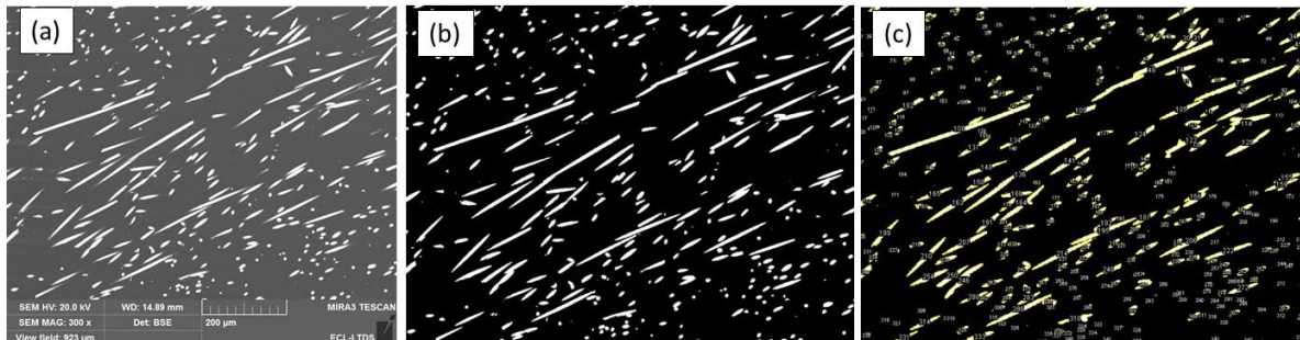
Fig. II. 25 Image analysis process: (a) obtained SEM image; (b) binarized image; (c) image showing particle analysis.
