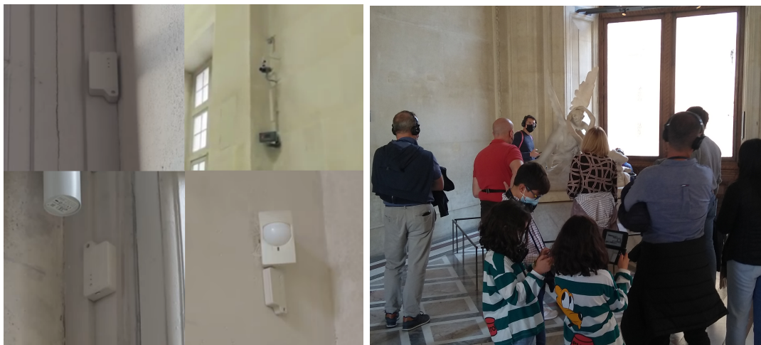
Bluetooth (smartphone app) and WiFi (Nintendo 3DS) beacons installed throughout the Louvre.
