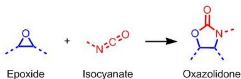
Scheme 4.1 - Oxazolidone group synthesis from epoxide and isocyanate.
