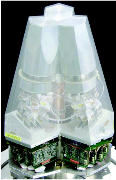
(b) Picture of a triplet mounted in a triple cryostat. The triplet cover is shown in semi transparency for greater clarity.
