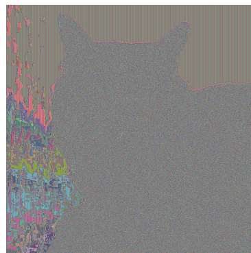
(b) The same picture, encrypted using AES-128 in ECB mode: the cat remains visible.
