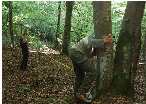
(c) Tree Crown extension measured with clinometer, compass, hypsometer and compass, and transponder. (d) Tree Crown extension measured with clinometer, compass, and ruban tape.
