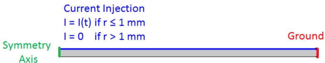
Figure 3-24 2D axisymmetric model: Electrical boundary conditions
