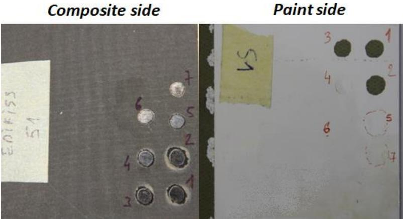
Figure 5-36 LASAT test results on CFRP+ECF+Paint(EDIFISS51)
