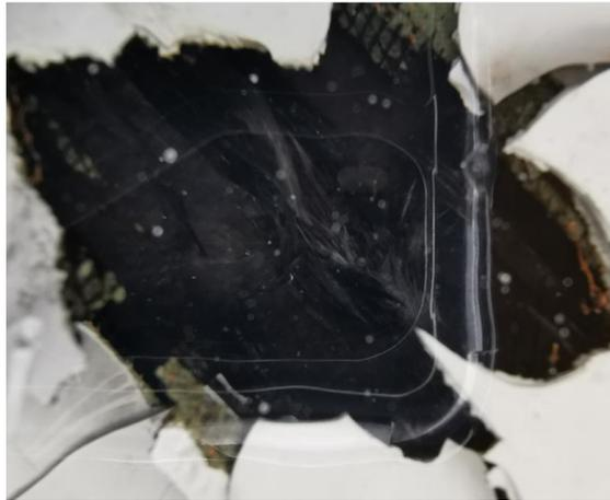
Figure 6-57 Internal damage study for severe configuration: CFRP (13plies) + ECF195 + 1000µm of paint: Top view
