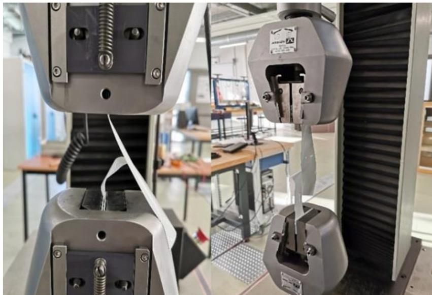
Figure 5-27 Tear trouser test set up (Left: Before test/Right: During test)
