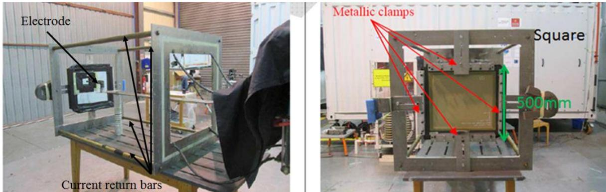
Figure 2-8 DGA-TA test set up example
