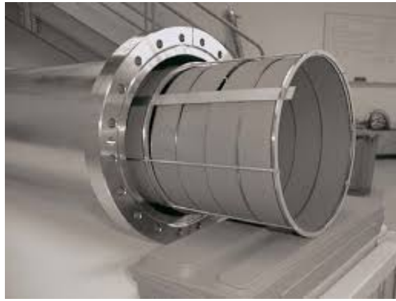
Figure 1.2. Schematic view of the St-707 total NEG pump [10].
