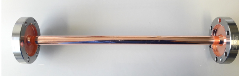
Figure 2.7. Electroformed chamber with the stainless steel flanges assembled using DC plating in the bath that contains a brightener.
