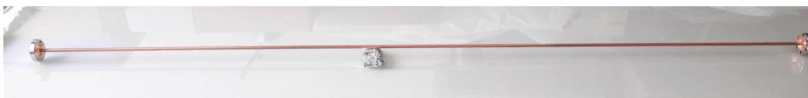
Figure 7.3. 5mm diameter, 1.2 meters length, NEG coated chamber.
