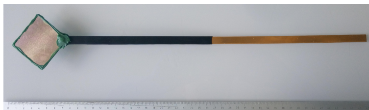
Figure 5.7. Platelets after copper PVD coating, before electroforming.
